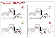
The STOPSAFE™ system for S5 cabrio avoids improper use of the machine. The system switches off the rotation if the rotor runs upwards and the hood is being opened. At the same time, if the hood is open it prevents the selection of the upward rotor direction.
