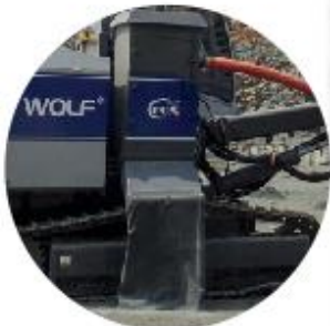
Dust Collector (primary and secondary)
