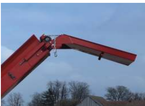
A slide with adjustable angle can be mounted to the ends of all belt conveyors, to allow processed wood fall further distances. Easily installed with 4 screws.
