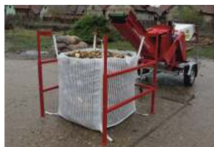
The dedicated big bag frame can be locked at two different heights. Either for logging with or without a pallet underneath the bag. The frame can be disassembled for easy transportation.
