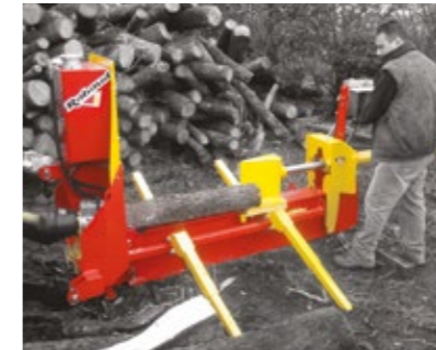
Log splitting with 1.15m clearance
