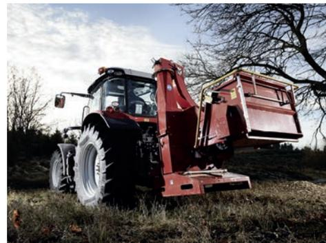
TP 250 PTO is equipped with a folding funnel with the operating bar hinged at the top. The ejector spout is rotatable (300 degrees).
