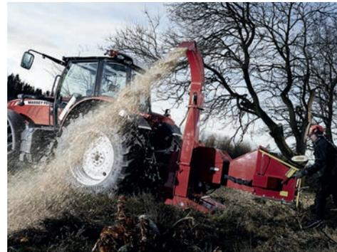
The end product is a first class quality wood chip from 4 to 13 mm. The chip size is hydraulically adjustable.
