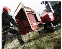
TP 130 PTO can also easily chip thin and soft branches - due to the short distance from the feed rollers to the blades and the position of both vertical and horizontal counter steel.
