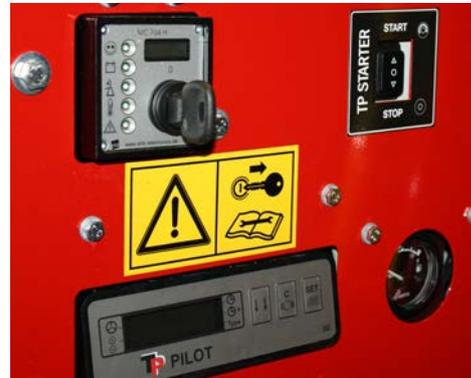
**TP STARTER:** Start-up can't be easier. Just turn the key and press the start button - you have started. The no-stress control **TP PILOT™** is the means to a smooth operation that prevents engine overload and allows you to read off disc rpm, working hours etc.
