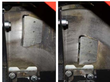
The 4 TP OPTICUT™ blades are placed alternately on the inner and outer part of the disc. This way, a blade is always engaging the wood, causing fewer vibrations, lower fuel consumption and a uniform wood chip.
